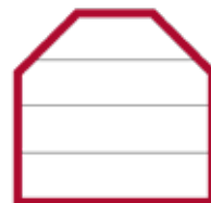
A spigoli obliqui Inclined-edge lintels
